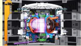
aims to transition from experimental studies of plasma physics to full scale electricity producing power stations. The goal is a tenfold return on energy (500 megawatts of fusion power from 50 megawatts of input power).
