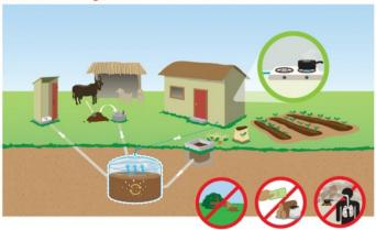
If implemented and maintained correctly, the process will provide the self -sustaining cycle we are working towards. The waste product is processed and the slurry used as fertilizer in the recently constructed Greenhouse. The methane byproduct can be harnessed as energy for cooking.
